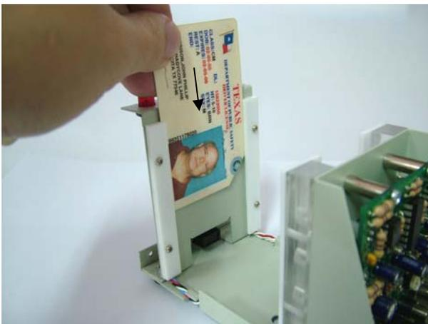
**Step B5** Drop the card again onto the card guide slot to ensure smooth entry of card by gravity without any force.
