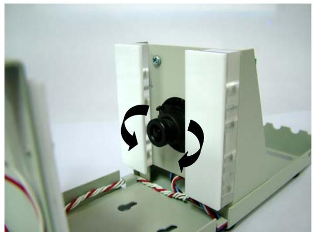
**Step F2** Turning the front knob on the camera clockwise or anti clockwise to achieve the sharpness required.
