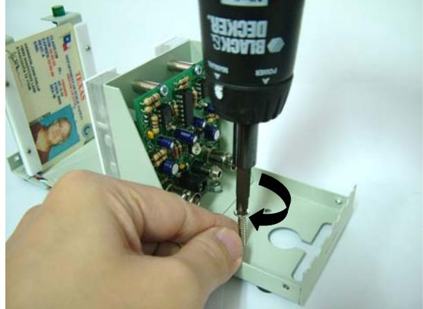
**Step A6** Prefer to drill a small hole on the location mark for easy mounting of the screws onto the surface.
