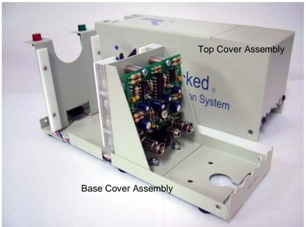
**Step A4** Top and base cover are separated as shown above.
