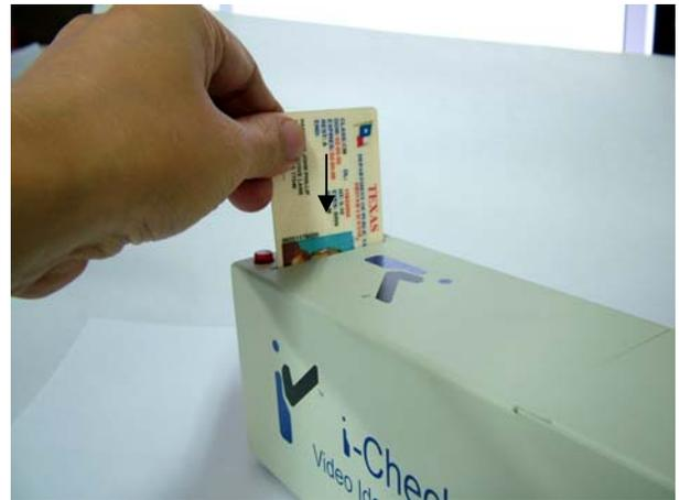
**Step B6** Slide on the top cover on the base cover assembly for confirmation of the card able to enter by gravity feed.
